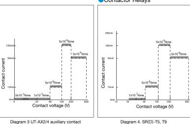
Note 1: The contact reliability indicates the failure rate  $\lambda$  60 (the number of failures/the number of opening and closing operations, per contact) at 60% reliability standard. This reliability is applied when the product is in use under a clean atmosphere in the standard specification environment (Refer to page 14).
