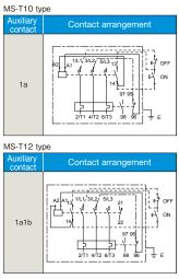
Note 1) The above figure gives an example of when the main circuit and operating circuit use the same power supply. The solid line is already wired. The dashed line and two-dot chain line sections must be wired.
