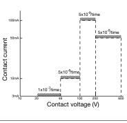
Diagram 2 S(D)-T, UT-AX11 auxiliary contacts
