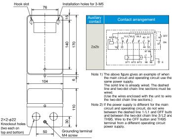
When mounting the MS-T10 to T21 types, leave 100mm of space below the box.
