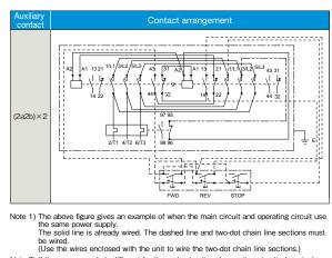
Note 2) If the power supply is different for the main circuit and operating circuit, do not wire between the dashed line 1/L1 and STOP button and between the two-dot chain line 3/L2 and TH95. Wire to the STOP button and TH95 terminal from a different operating circuit power supply.
